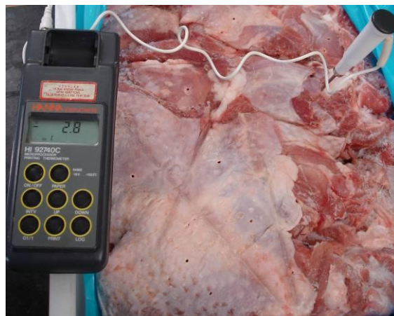
Turkey filets, 40 kg (2 x 20 kg) 320 - 360 kg/h capacity for a final temperature between -4 °C and -2 °C or 250 - 290 kg/h capacity for a final temperature between -3 °C and -1.5 °C
