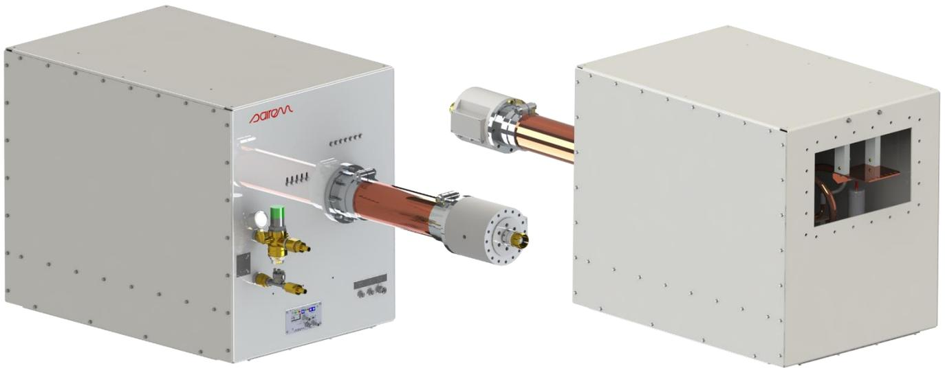
The matching box (MB) matches the impedance between the 50  $\Omega$  line from the generator and the impedance of the applicator, which is generally capacitive and very low resistive impedance. Two adjustable capacitors are used to match tune and load; depending on the load, a cooling coil is integrated to compensate the capacitive part of applicator; capacitors are motor-driven.
