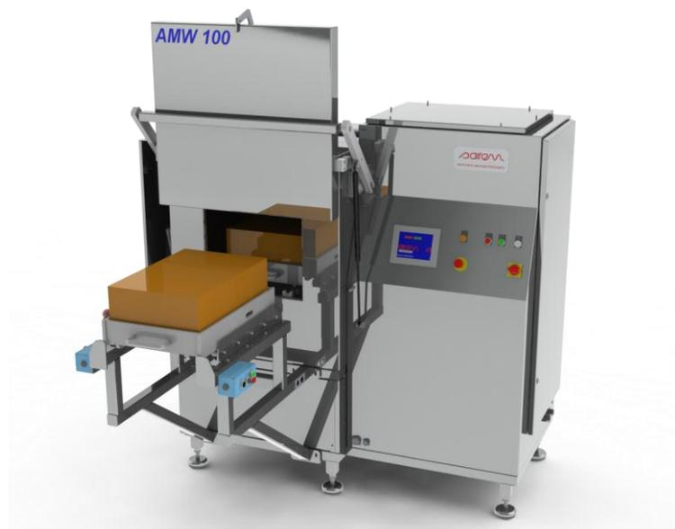
The Labotron 915 AMW 100 is a 915 MHz, 5 kW, laboratory batch oven using microwave heating with main applications in food processing, e.g. thawing, pre-cooking, cooking, drying, pasteurization, disinfestation, etc. It can also be used for other materials such as wood, rubber, textile, composite materials...
