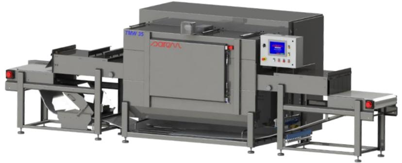
The very low floor space, the length under microwaves (residence time) and the crossed coupling of microwaves above and below the blocks, are a few examples of the solutions used to conciliate capacity, flexibility, efficiency and homogeneity.
