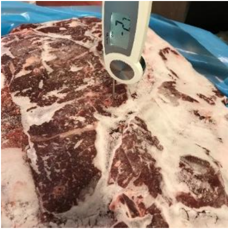
Beef 25% fat, 50 kg (1 x 25 kg) 190 kg/h to 210 kg/h from -18 °C to -6 °C/-4 °C
