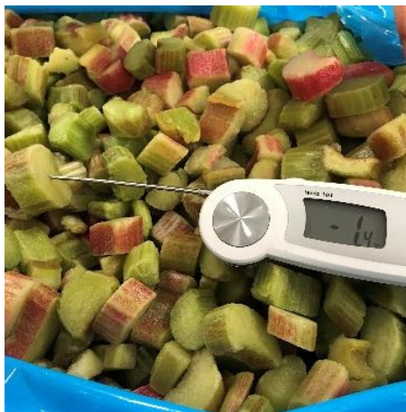
Rhubarb in 10 kg blocks (1 x 10 kg) Capacity: \approx 100 kg/h from -18 °C to -3 °C/-1 °C
