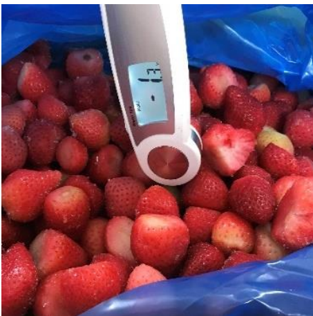
Strawberries in 10 kg blocks (1 x 10 kg) Capacity: \approx 100 kg/h from -18 °C to -3 °C/-1 °C
